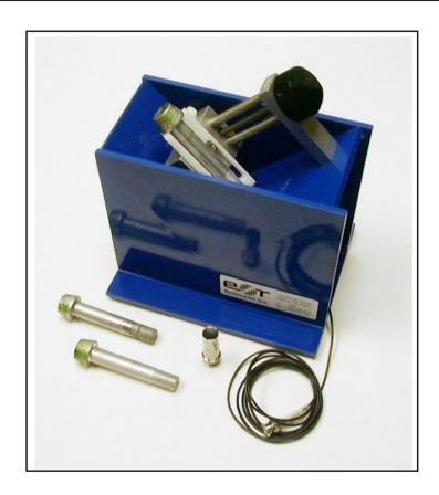
The Ultrasonic Bolt Inspection System is a mechanical fixture for manual immersion ultrasonic inspection of bolts for cracks in the thread, shank or head-to-shank fillet. Its primary application is the nondestructive inspection of aircraft wheel tie bolts. It is also used for testing of automotive parts and other cylindrical components for voids, inclusions and weld integrity.
